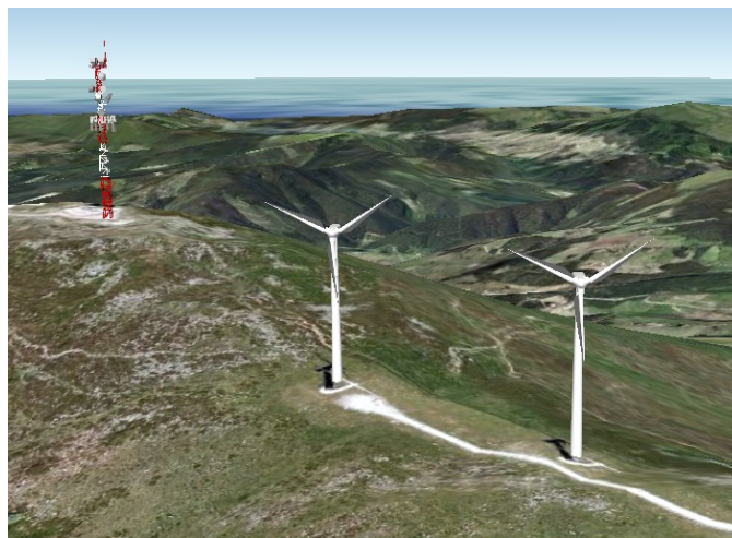
Fig. 1. Example of a “Preview Study” on Google Earth, showing a television tower and two wind turbines
