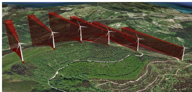
Fig. 4. Example of Wi^2 result for shadowing on target detection: volume where the radar beam is obstructed by each wind turbine.
